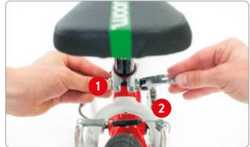
**Closing:** With open clamping lever in one hand, turn the adjusting nut in a clockwise direction while holding the clamping lever with the other hand. Now tighten the nut. Then turn the clamping lever using the palm of your hand in a manner that you can see the outer side of the lever.
