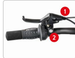
Some time after starting to use the brake and its regular use, you will notice some stretching of the brake cable. The **adjustment screw** serves the purpose of minimal adjustment.
