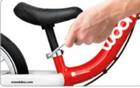
For the woom 1, 1 PLUS and 2 the height of the seat can be adjusted by opening the seatpost clamp with a hex key.
